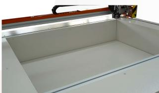
Lift table to load from the top layers of material to be glued (for over 400 mm in height), that automatically rise and position at the required working height at the end of each single operation
